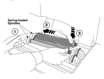
Note: Make sure that you load the spools with the proper orientation—that is, with the receive spool (empty when new) in the front. The supply spool is identified by a black ring on the left side.
