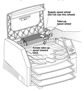
Note: Do not use the supply spool (rear) wheel to take up ribbon slack. This would cause spent ribbon to be reused.
