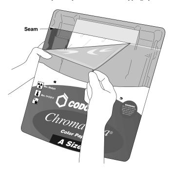
**CAUTION:** Do not remove the printed cassette cover; it protects the media from dust and other contaminants. Always hold and store the cassette with the open side up to prevent the sheets from falling out.
