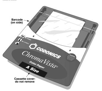
Each cassette contains a barcode that identifies the media type and size, serial number, and sensitometry information. The cassette's lot number and "Use by" date are also printed on the barcode label.
