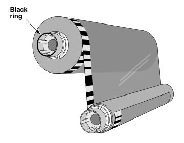
6. To take up any ribbon slack, rotate the top of the take-up spool's wheel (that is, the front wheel) towards the back of the imager, as shown in the following figure.
